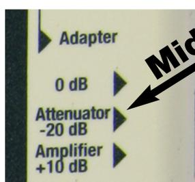
When the attenuator is connected, set the "Adapter" switch of the HF-Analyzer to "Attenuator -20 dB" (See picture on left). This activates the integrated automatic conversion feature of the HF-Analyzer. The true signal strength value can be read from the display without any manipulation. The vertical line on the left side of the display indicates the correct measuring unit.
